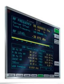
The R&S°FS-K15 option measures the most important parameters of VOR and ILS signals such as VOR phase, ILS DDM as well as the modulation depth and frequency of the individual signal components. When the option is integrated into the R&S°FSMR measuring receiver, the complete calibration and verification of VOR/ILS generators or generator parts of air navigation testers is easy – no additional equipment required.
